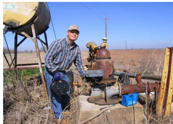
POSGCD staff uses an E-line to measure the water level in this irrigation well in the Brazos River bottom.
