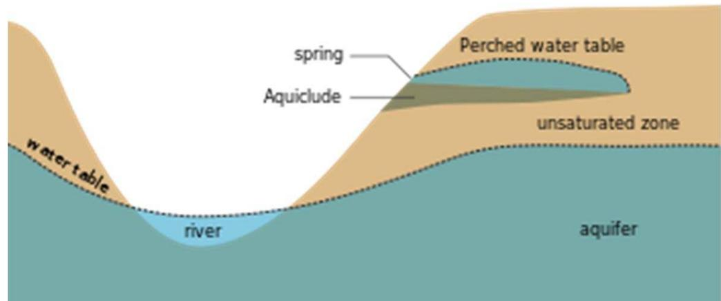
**Schematic of a spring connected to a perched water table
