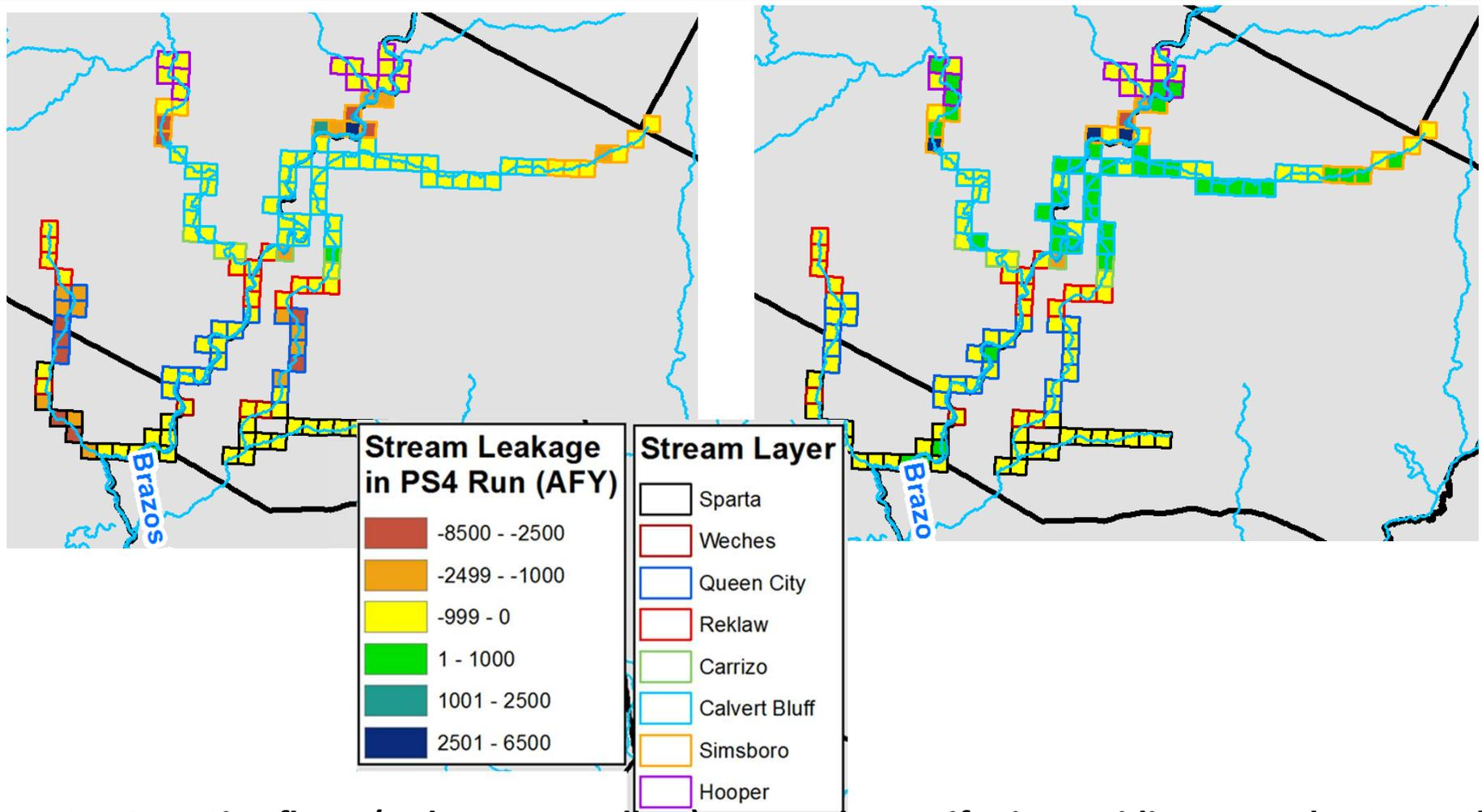
**Note: Negative flows (red, orange, yellow) means the aquifer is providing groundwater to the stream – so stream is gaining. Positive flows (greens and blues) means the aquifer if receiving water from the stream – so stream is losing.**
