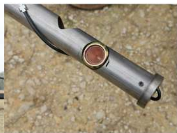
Recently, POSGCD converted an abandoned oil well to a monitor well in the Hooper Aquifer. Shaped charges were used to perforate the casing at the appropriate depth.
