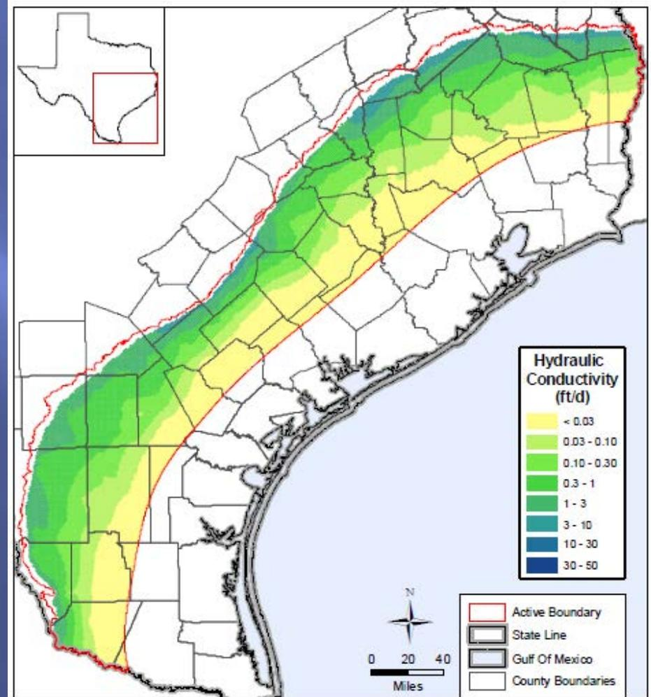
Figure 8.1.5 Horizontal hydraulic conductivity in feet per day of the Lower Yegua Unit subcrop.
