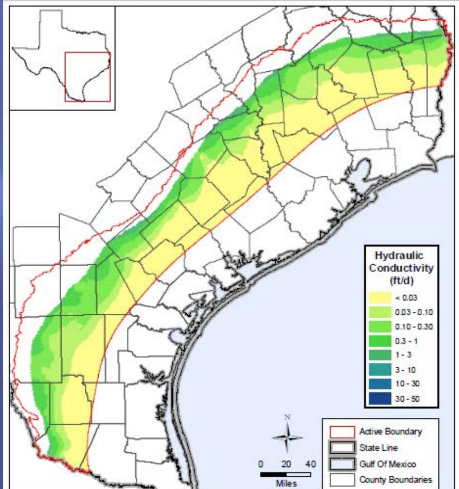
Figure 8.1.3 Horizontal hydraulic conductivity in feet per day of the Lower Jackson Unit subcrop.
